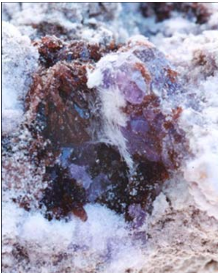
Figure 5. Purple coquimbite crystals associated with halotrichite (acicular white) and römerite (dark brown), embedded in sugary-white coquimbite. Field of view is 2 cm.
