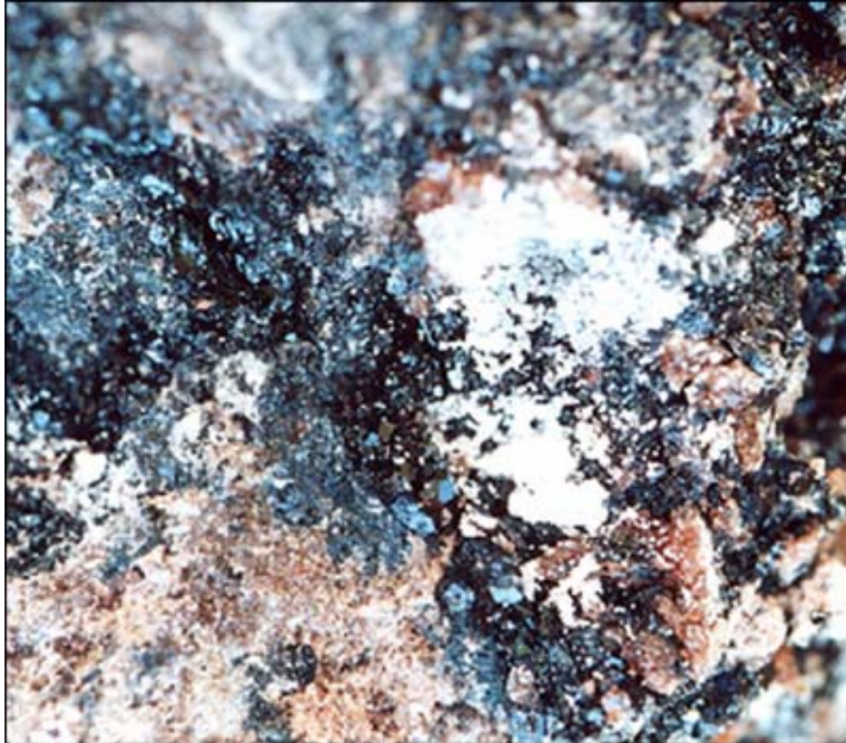
Figure 20. Typical 1-cm specimen of voltaite showing the black cubic form associated with brown römerite and halotrichite.
