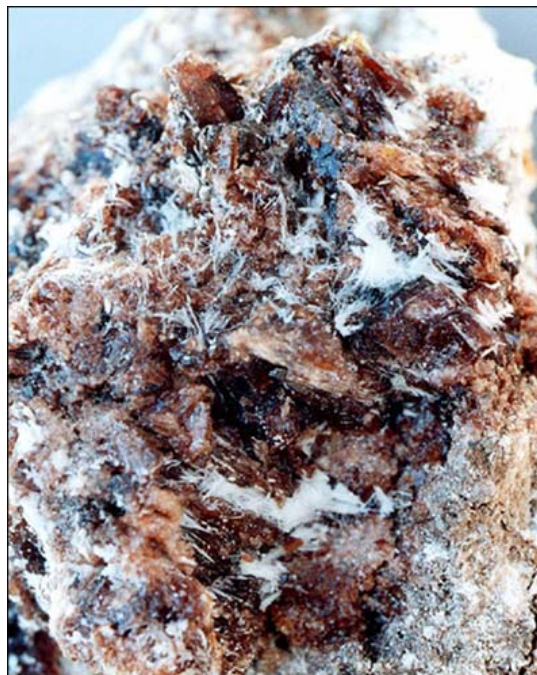
Figure 19. Typical specimen, 2 x 5 cm, of dark brown römerite with white fibrous halotrichite.
